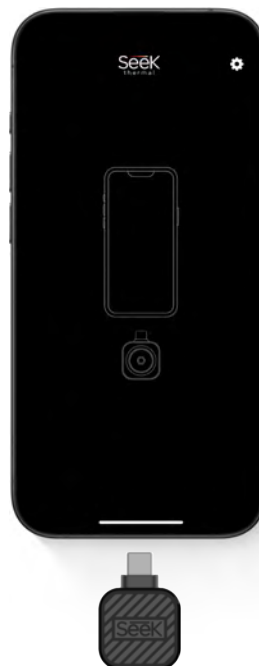
2. Connect the camera to your device
