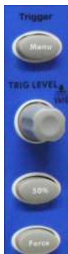
Fig. 13 Trigger Control Zone
