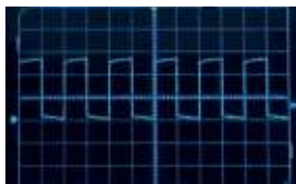
INCORRECTLY SET COMPENSATION
