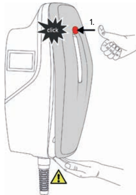
Fig. 18: Attach front cover (example) - 1
