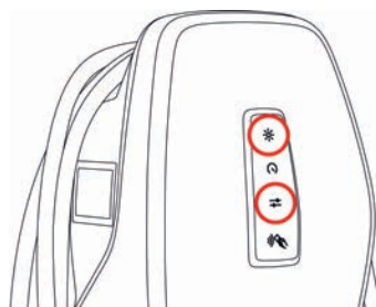
Fig. 11: Activate access point (example)
