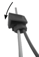
Figure 6: Closing the safety clamp
