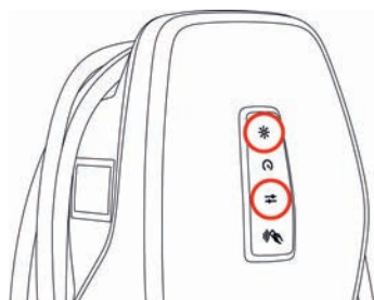
Fig. 12: Activating the access point
