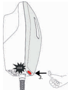
Fig. 16: Attach front cover - 2
