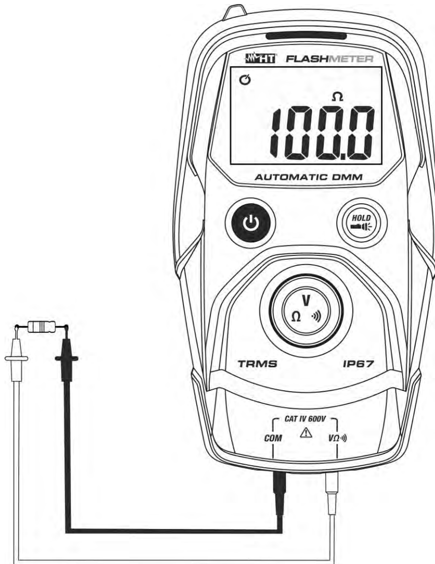
Fig. 5: Use of the instrument for Resistance measurement
