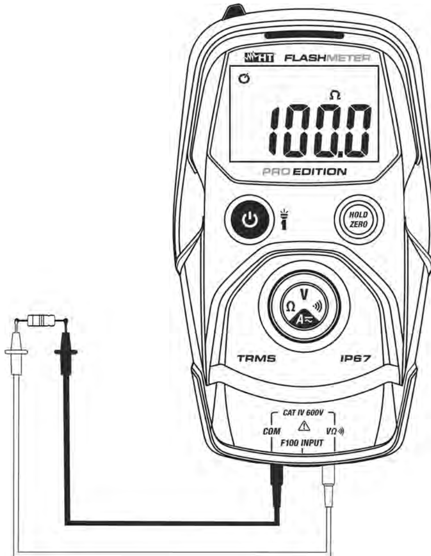
Fig. 5: Use of the instrument for Resistance measurement
