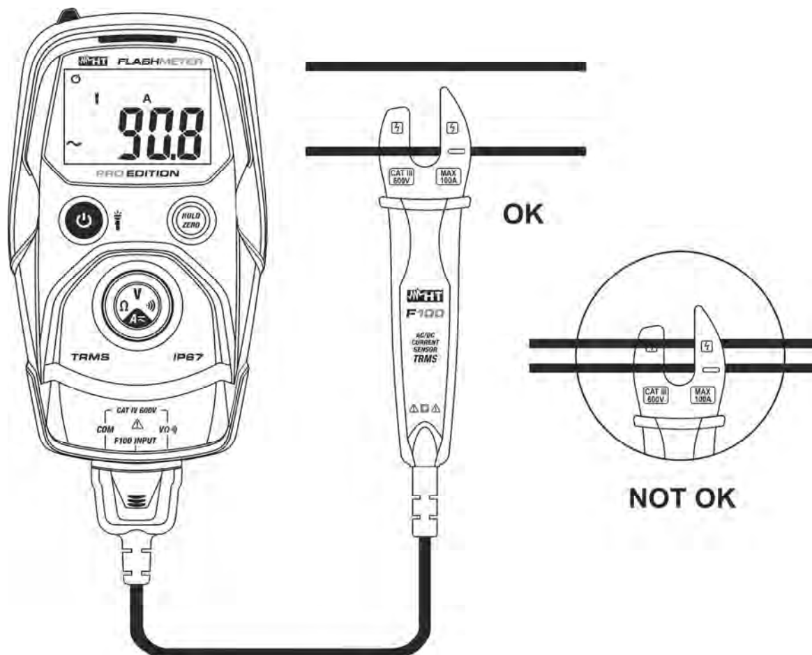
Fig. 7: Use of the instrument for AC/DC Current measurement
