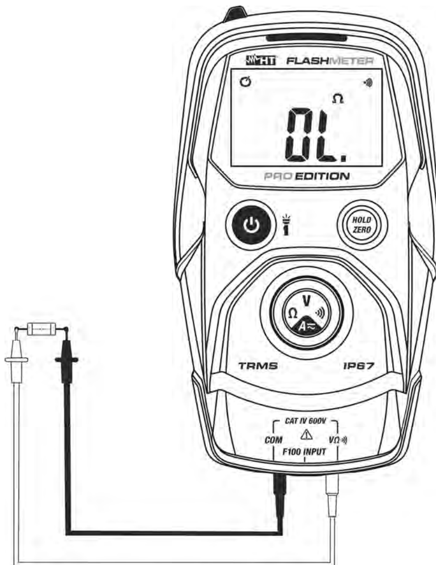
Fig. 6: Use of the instrument for Continuity test
