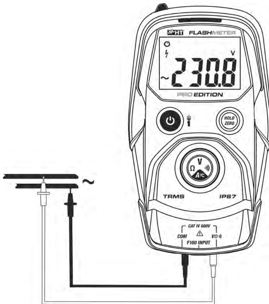
Fig. 4: Use of the instrument for AC Voltage measurement
